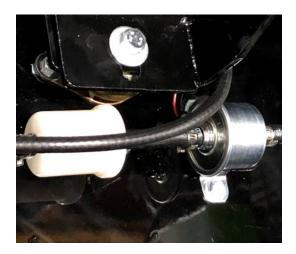
3. Disconnect the temperature sensor. If the engine starts with the temperature sensor disconnected the temperature sensor is bad. Replace it. 4. Disconnect the oil pressure sensor. If the engine starts with the oil pressure sensor disconnected and the oil level is good, the oil pressure sensor is bad. Replace it.
