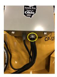
3. Check FU1 Fuse inside the control box. If the fuse is bad replace it. If the fuse keeps blowing, check heated hose trigger switch wiring for a short. If the problem persists, call Sealmaster. [800] 395-7325
