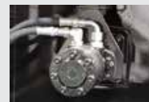
Hydraulically Driven Full Sweep Agitation
