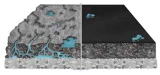
MasterSeal replenishes the binder that is lost through weathering and aging and provides a barrier to moisture intrusion as well as ultraviolet rays, chemicals and salt. MasterSeal beautifies pavement, enhancing the image and curb appeal of commercial properties, home driveways, roadways and more.
