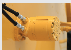
Direct-Drive FWD/REV Full Sweep Agitation
