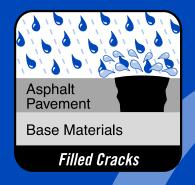
Filling cracks with Crack Filler helps prevent rain and moisture from flowing through the pavement and causing erosion or failure.
