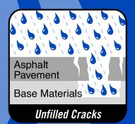
Left unfilled, cracks will allow rain and moisture to flow through pavement and erode base materials ultimately resulting in potholes and pavement failure.
