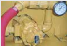
Positive Displacement Material Pump
