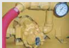
Positive Displacement Material Pump
