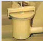
Easy Access Basket Strainer Reduces Tip Clogging
