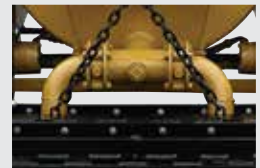
Dual Easy-Open Butterfly Sealer Discharge Valves
