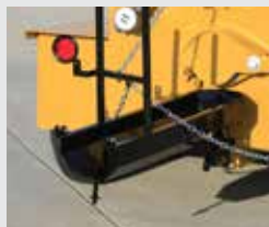
Heated Adjustable Locking Chute
