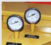
Oil and Material Temperature Gauges
