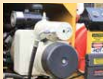
Direct Drive Air Compressor
