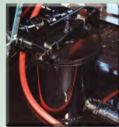
Easy Access Basket Strainer Reduces Tip Clogging
