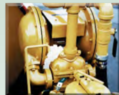
Hydraulically Driven Dual Diaphragm Material Pump
