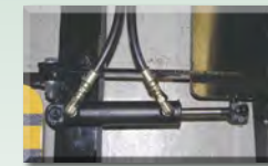
Hydraulic Shift Option for Angling the Squeegee
