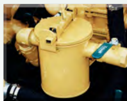
1-Gallon Basket Strainer Reduces Tip Clogging
