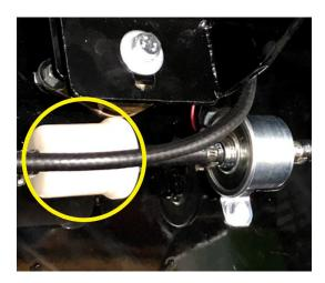
3. Disconnect the temperature sensor. If the engine starts with the temperature sensor disconnected the temperature sensor is bad. Replace it.
