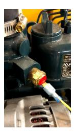
4. Disconnect the oil pressure sensor. If the engine starts with the oil pressure sensor disconnected and the oil level is good, the oil pressuresensor is bad. Replace it.
