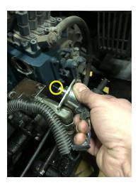
6. Ensure the ground wire is also free of rust and corrosion. An improper ground could cause the solenoid to malfunction.
