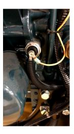
5. Disconnect the fuel shutoff solenoid. Hold the solenoid against something metal for ground. Turn the key switch on and crank the engine momentarily. If the plunger pulls back into the mechanism the solenoid is good. If not, it needs to be replaced.
