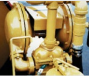
Hydraulically Driven Dual Diaphragm Material Pump
