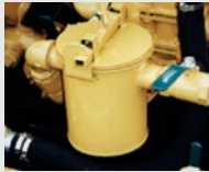
1-Gallon Basket Strainer Reduces Tip Clogging
