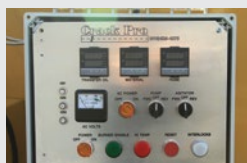
Digital Control Center with protective steel cover
