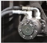
Hydraulically Driven Full Sweep Agitation
