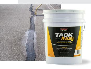
**APPLICATION INSTRUCTIONS:** Gently stir Tack Away prior to use. Fill Garden-type, hand-held pump up sprayer with Tack Away. Adjust spray tip to a medium fan pattern. Spray Tack Away directly on freshly applied crack sealant while minimizing overspray onto pavement.
