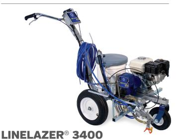
The LineLazer 3400 features new easy reach controls, new handle bar design with comfort grips, higher output and higher maximum pressure, new electronic pressure control, and new easy-roll wheel design. Swivel front wheel. Parking brake to prevent striper from rolling on uneven surfaces.
