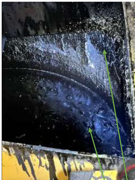
FLAKES IN MATERIAL FROM BUILDUP
