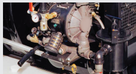
Air Driven Dual Diaphragm Pump with Basket Strainer
