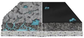
PMM replenishes the binder that is lost through weathering and aging and provides a barrier to moisture intrusion as well as ultraviolet rays, chemicals and salt. PMM beautifies pavement, enhancing the image and curb appeal of commercial properties, home driveways, roadways and more.
