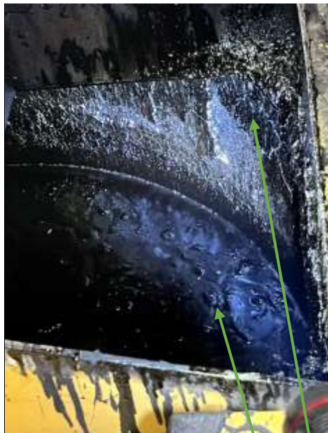
FLAKES IN MATERIAL FROM BUILDUP
